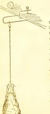
This represents a model of a Chimney Screw-jack for suspending joints to. Its cost is very trifling, and may be purchased at any ironmonger's. It will fit on any mantel-shelf; and it enables the joint to be shifted nearer or further from the fire, as occasion requires.
